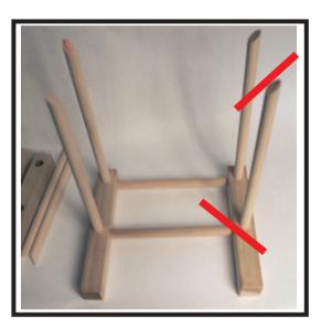
Glue **long rails** into **legs**, be sure 45° angle is placed as shown to match up with **short rail** cut.
