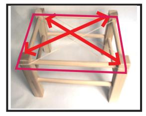
Use elastics to hold stool together until dried, either between corners or around all 4 legs (depends on size of your elastics) Finish stool as desired when dry (paint, oil, stain)
