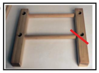
Glue **short rails** into **legs** as pictured. be sure 45 degree cut is facing UP in hole. **Long rail** will meet up at 45° inside leg. Do both sets of **short rails**
